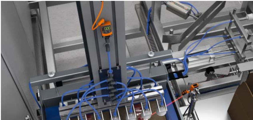
Vacuum pressure sensor for measuring the vacuum on a suction gripper
